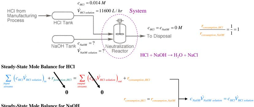
$$\sum_{\substack{input \\ streams}} \left( c_{NaOH} \dot{V}_{NaOH \ solution} \right)_{in} + r_{formation, NaOH} = \sum_{\substack{output \\ streams}} \left( c_{NoH} \dot{V}_{NaOH \ solution} \right)_{out} + r_{consumption, NaOH} - \dot{V}_{NaOH \ solution} = \frac{c_{HCl} \dot{V}_{HCl \ solution}}{c_{NaOH}}$$
