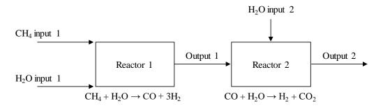
For the Reactor 1, the methane steam reforming reaction occurs  $(CH_4 + H_2O \rightarrow CO + 3H_2)$ . The methane input flows into the Reactor 1 at a rate of 64.2 g/min. Water input enters the Reactor 1 in a separate stream. The amount of water entering the Reactor 1 is 25% more than that needed to react stoichiometrically with all of the entering methane. The conversion of methane in Reactor 1 is 75%.
